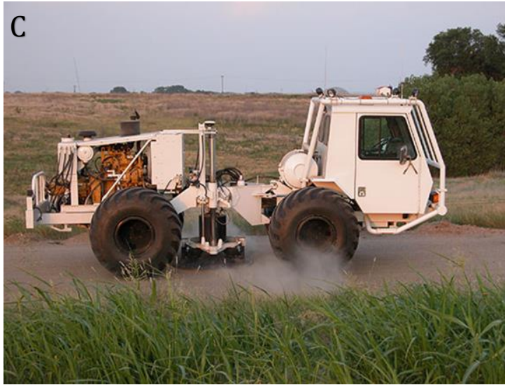
Figure 3: Seismic surveying process and potential impacts. (A) Showing an animated Vibroseis process, (B) Showing a real life Vibroseis process, (C) Showing minimal dust generated from the process, (D) Showing minimal vegetation impact associated with a new access path (transect route), and (E) Showing the weight drop alternative method.
